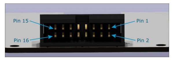
The picture above shows the connector on top view and the official pin numbering for IDC jacks. Please keep in mind that the pin numbering for the female socket is mirrored (!).
