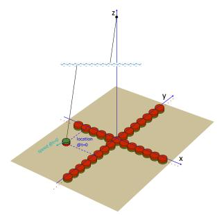
The ball is represented by an infinite small magnet at the end of a long fiber. The fiber is fixed on  $(0;0; \rightarrow \infty)$ ; the magnet hovers shortly above the xy-plane.
