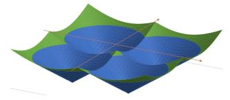
Based on the simplification above, the 3Dmap of the static forces shows the steady state operating points clearly: one by quadrant.
